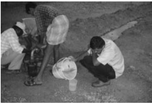
Photo 3. Water measurement during technical evaluation of drip system in Tumkur, Karnataka
